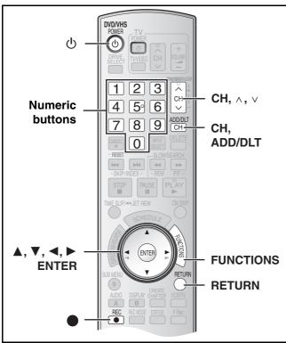
After plugging the unit into your household AC outlet and pressing [ $\dot{\oplus}$ , DVD/VHS POWER] to turn the unit on for the first time, the unit assists you to set the on-screen language, and automatically tunes in all the channels it can receive and sets the clock.
